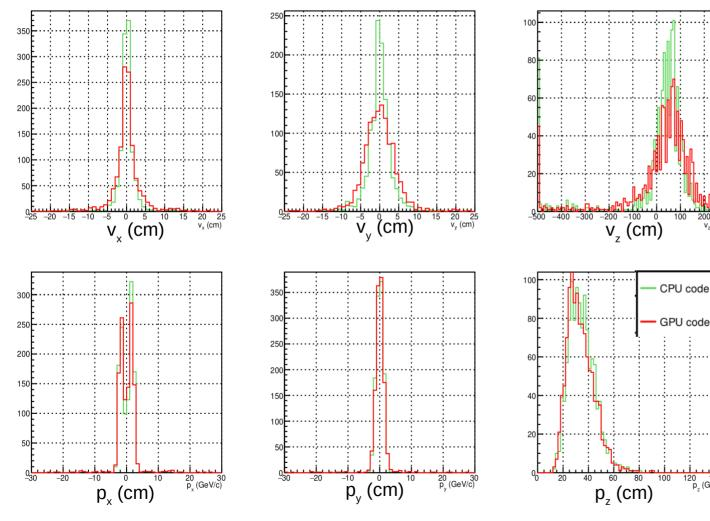
Pure Monte Carlo dimuons: Green: analysis made with CPU track reconstruction Red: analysis made with GPU <sup>200</sup> 300 v<sub>z</sub> (cm) track reconstruction
