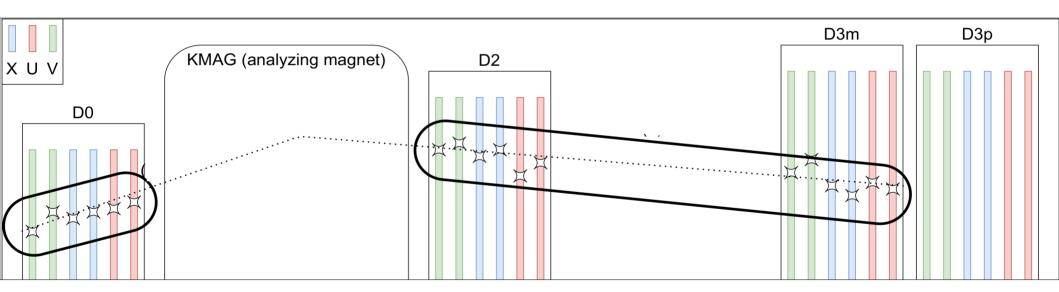
X: vertical wires U: wires at +14 degrees with respect to x wires V: wires at -14 degrees with respect to x wires
